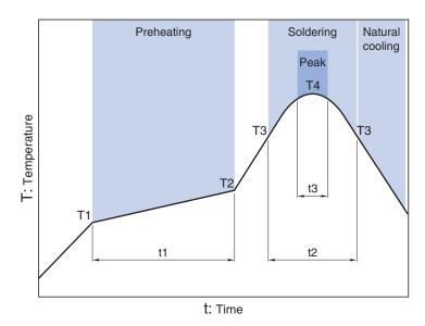
Soldering Preheating Peak Temp. Temp. Temp. Time Time Time T1 T2 T4 Т3 t3 150°C 180°C 60 to 120s 230°C 250 to 260°C 30 to 60s 10s max.
