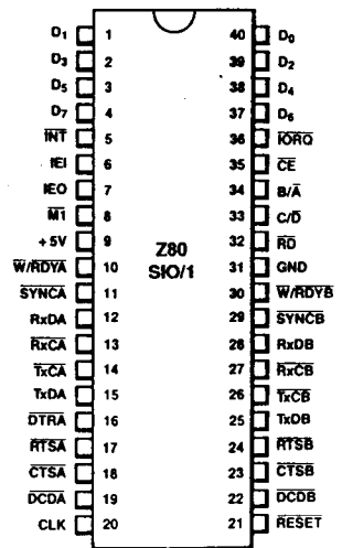
Figure 4. 40-pin Dual-In-Line Package (DIP), Pin Assignments
