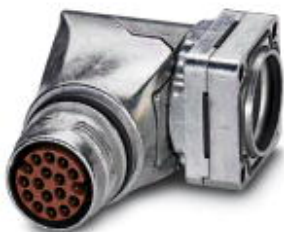
Device connector, front mounting, angled rotatable, SPEEDCON locking, M17, number of positions: 17, type of contact: Pin, Crimp connection, Axial O-ring, 4x Ø2,7, shielded: yes, flange dimensions: 25 mm x 25 mm
