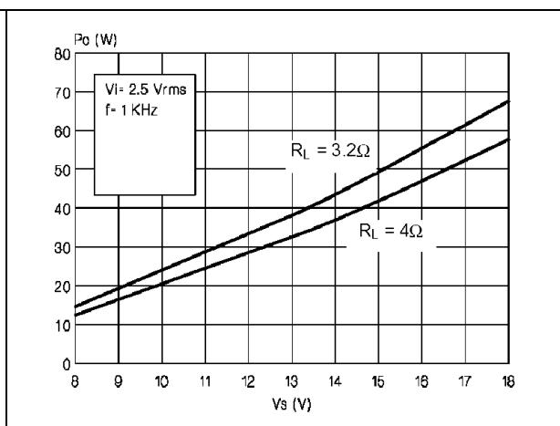
**Figure 6. Output power vs. supply voltage (@ $R_L = 4\Omega$ )**
