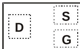
Top View Package Pin Configuration
