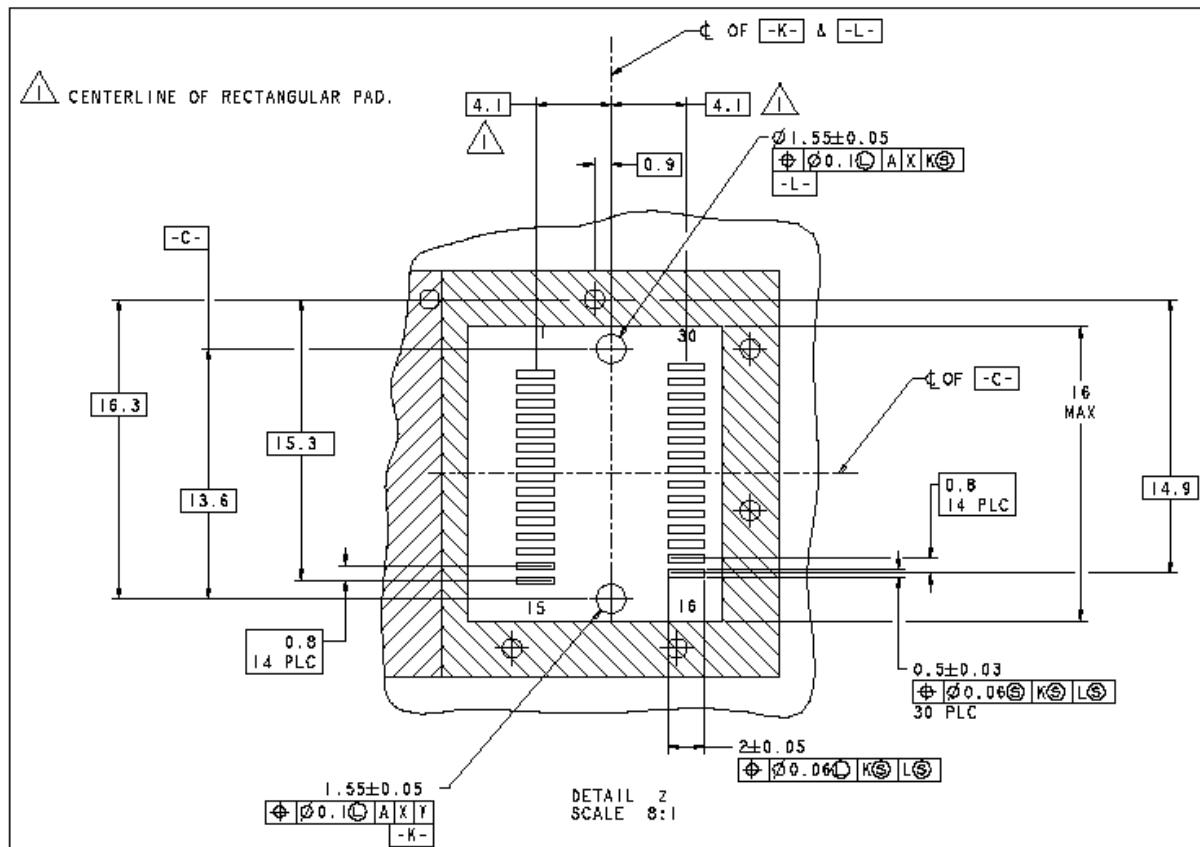
**XFP Detail Host Board Mechanical Layout (dimensions are in mm)**
