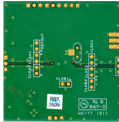
**Figure 4. Evaluation Board bottom View (Bare PCB)**
