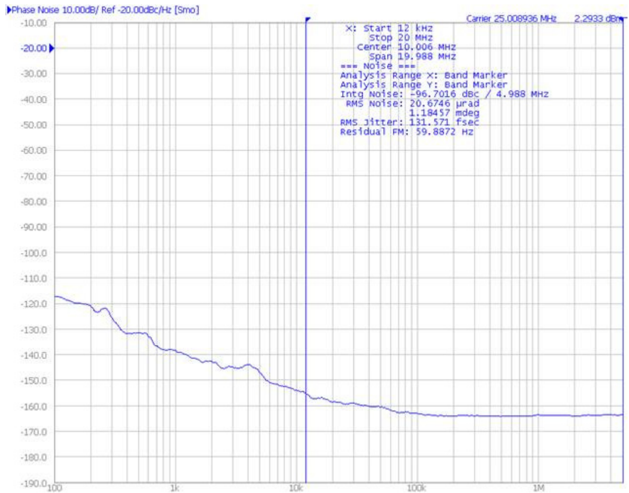
Figure 8. NB3N853531E Phase Noise with 25 MHz Crystal
