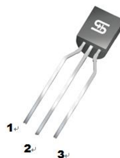
1. Collector 2. Base 3. Emitter TO-92 Plastic Package
