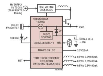
Figure 1. LTC3557/LTC3557-1 Simplified Typical Application
