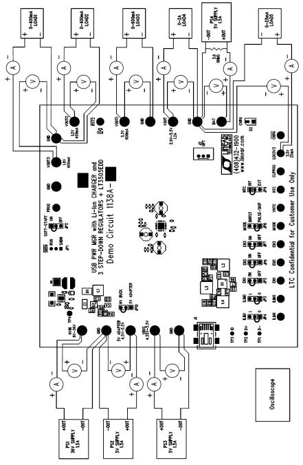
Figure 2. Proper Equipment Setup for DC1138A-A/B
