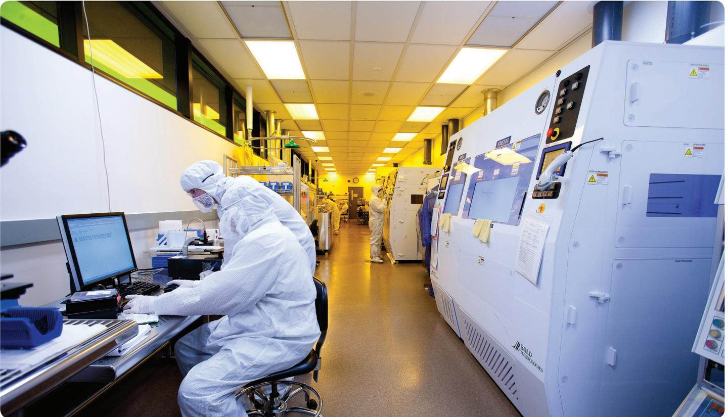
Merit Sensor owns and operates a MEMS wafer fab, which enables the production of customized piezoresistive pressure sensors for medical, industrial, and automotive applications. We help you get to market quickly with creative and flexible solutions and provide prompt, personal, and professional customer support.
