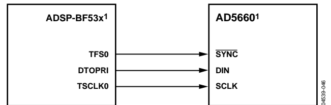
Figure 46. AD5660-to-Blackfin ADSP-BF53x Interface
