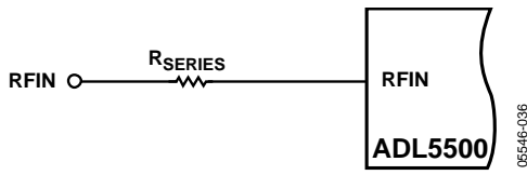
Figure 36. Attenuating the Input Signal
