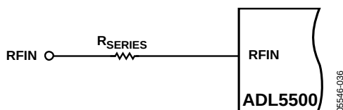
Figure 36. Attenuating the Input Signal
