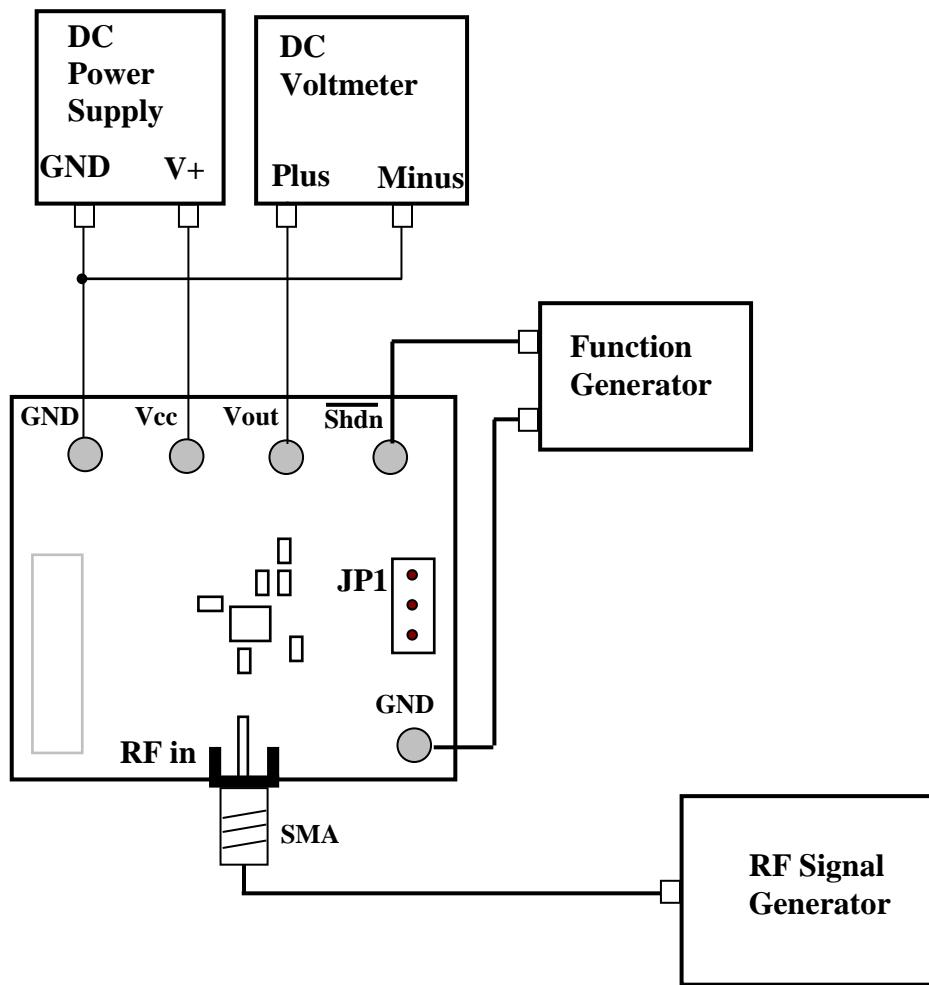
**DC539B Demo Board Connection Diagram**
