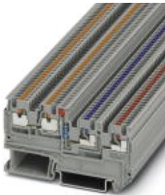
Sensor/actuator terminal block, Connection method: Push-in connection, Cross section: 0.14 mm 2 - 1.5 mm 2 , AWG: 26 - 14, Width: 3.5 mm, Color: gray, Mounting type: NS 35/7,5, NS 35/15
