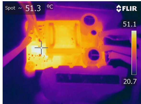
Figure 15. Thermal Image of the ADP1071-1 at 48 V DC Input, Full Load, No Airflow, and 0.5 Hour Soaking Time
