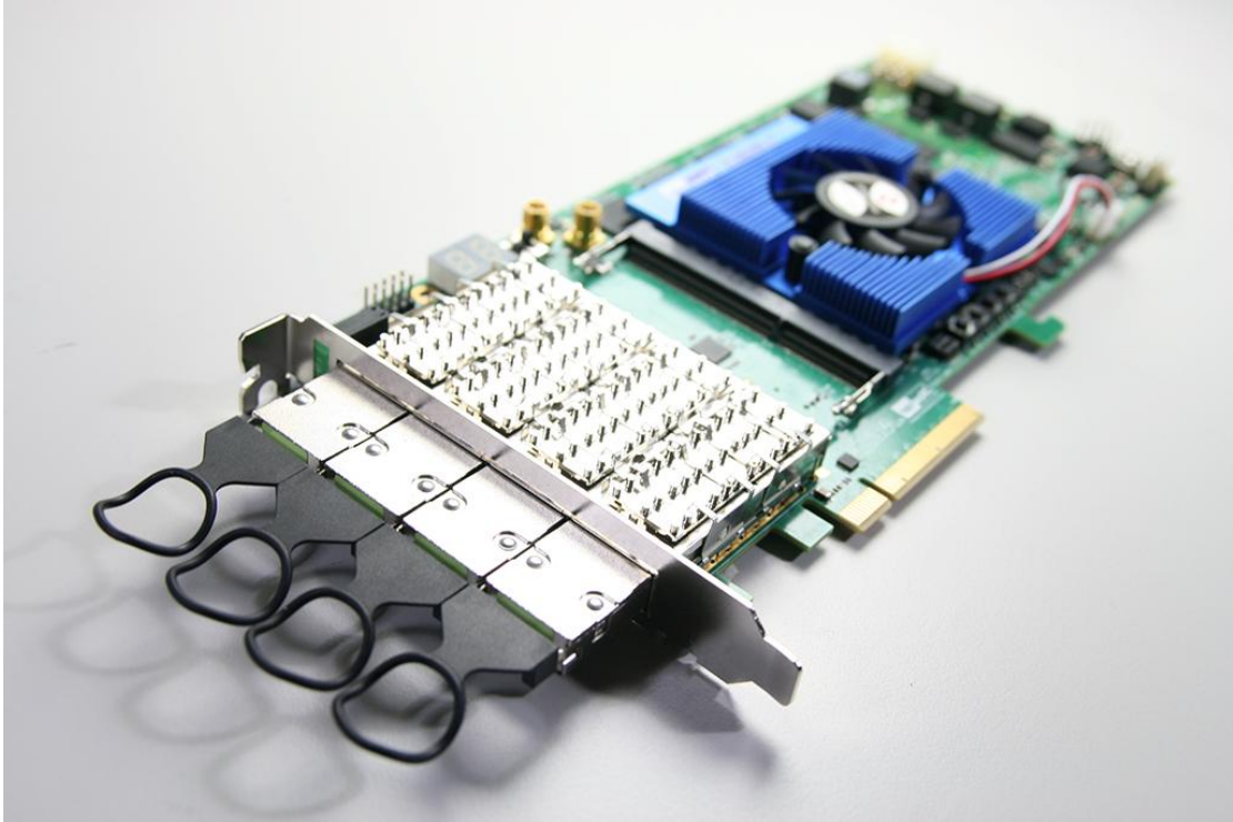
Figure 8-4 Four QSFP+ Loopback Fixtures Installed
