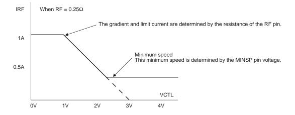
The current flowing to the motor and the control characteristics are determined by adjusting the resistance of the RF resistor.
