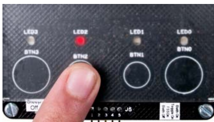
1. Touch a button; LED turns on
