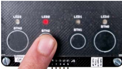
1. Touch a button; LED turns on
