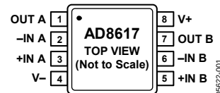
Figure 2. 8-Lead MSOP and 8-Lead SOIC_N
