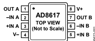
Figure 2. 8-Lead MSOP and 8-Lead SOIC_N
