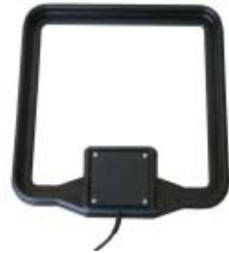
This antenna is a single-loop transmit/receive antenna with pre-set matching electronics for a transmitter frequency of 13.56MHz and impedance of 50Ω.
