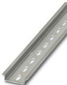
DIN rail, material: Steel, perforated, height: 7.5 mm, width: 35 mm, length: 1 m
