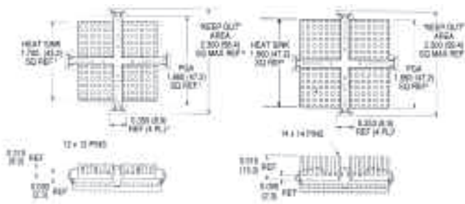
Dimensions: in. (mm) 649-33AB SPIDERCLIP™ ASSEMBLY
