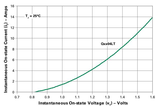
**Figure 3: On-State Current vs. On-State Voltage (Typical) (6A to 15A)**
