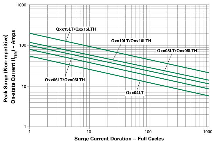
Supply Frequency: 60Hz Sinusoidal
