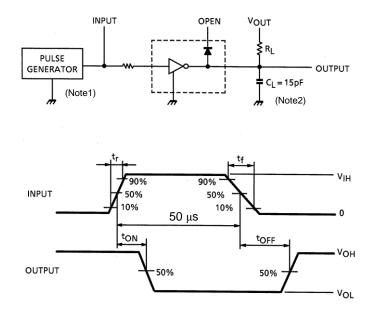
Note 1: Pulse width 50  $\mu s,$  Duty cycle 10%
