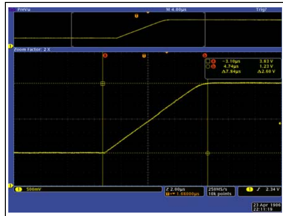
FIGURE 2-38: Half-Scale Settling Time (10h to 30h), V_{DD} = 5.0\text{V} , V_{REF} = 5.0\text{V} , R_L = 5\text{k}\Omega , C_L = 200\text{pF} (Time scale = 2\text{ }\mu\text{s} / \text{div} ).
