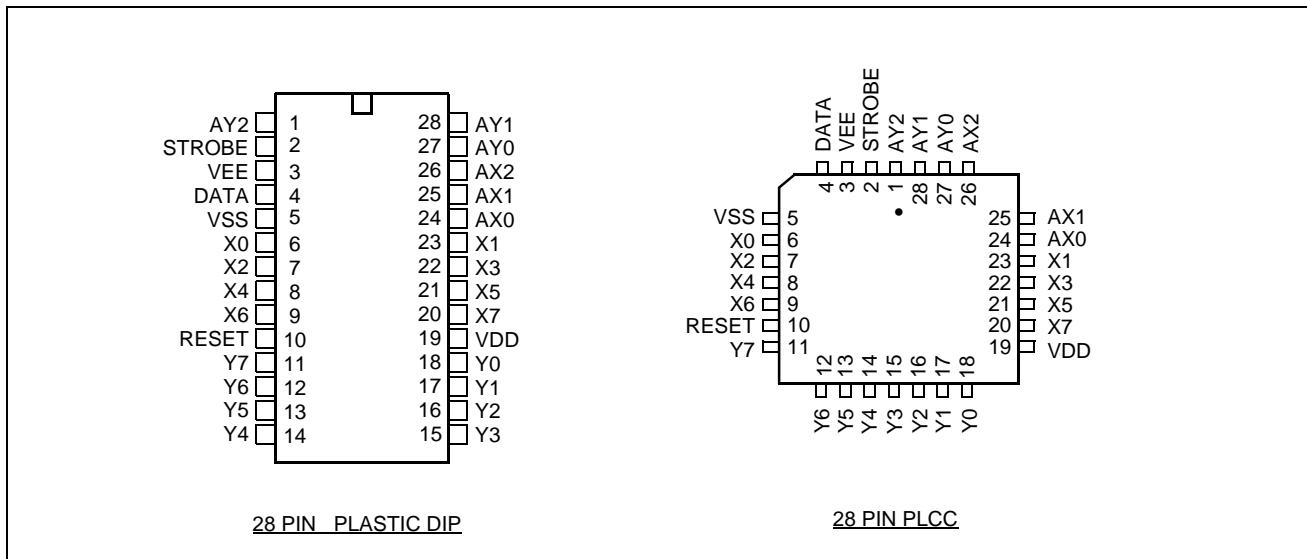
**Figure 2 - Pin Connections**
