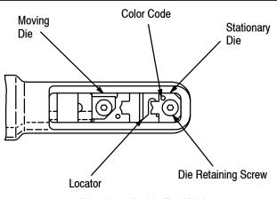
Dies Installed in Tool Yoke
