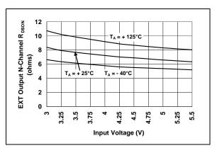
**FIGURE 2-12:** EXT Output N-channel R<sub>DSON</sub> vs. Input Voltage.
