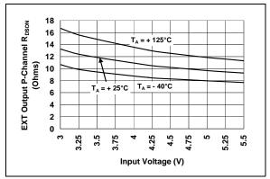
**FIGURE 2-13:** EXT Output P-channel R<sub>DSON</sub> vs. Input Voltage.
