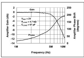
**FIGURE 2-3:** Error Amplifier Frequency Response.
