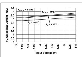
FIGURE 2-2: Input Quiescent Current vs. Input Voltage.
