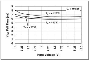
**FIGURE 2-8:** V<sub>EXT</sub> Fall Time vs. Input Voltage.
