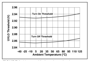
**FIGURE 2-11:** Undervoltage Lockout vs. Temperature.
