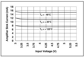
**FIGURE 2-5:** Error Amplifier Sink Current vs. Input Voltage.
