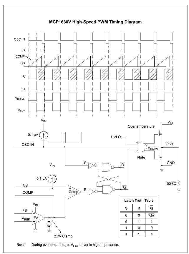
FIGURE 4-2: Cycle-by-Cycle Timing Diagram (MCP1630V).
