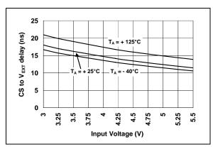
**FIGURE 2-9:** Current Sense to  $V_{EXT}$  Delay vs. Input Voltage (MCP1630).
