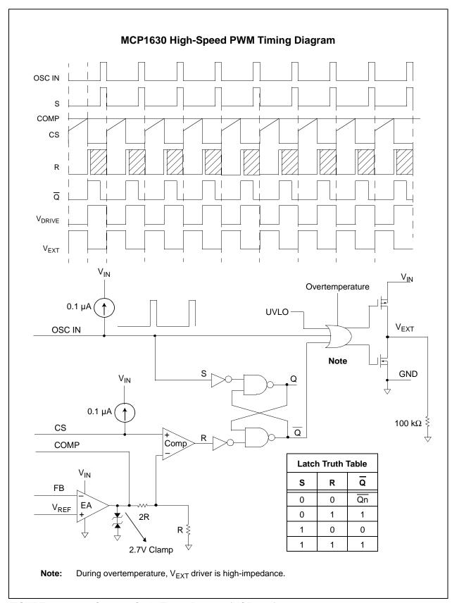
FIGURE 4-1: Cycle-by-Cycle Timing Diagram (MCP1630).
