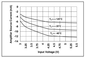
**FIGURE 2-6:** Error Amplifier Source Current vs. Input Voltage.
