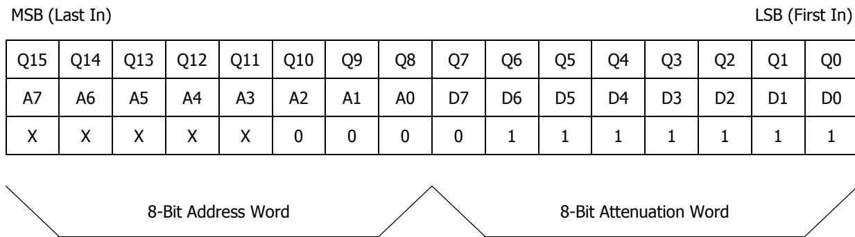
**Figure 3 -Default register settings set for Max Attenuation and 000 Address Word****REGISTER TIMING DIAGRAM: (NOTE THE TIMING SPEC INTERVALS IN BLUE)**
