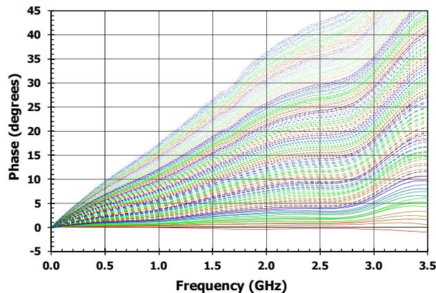
**Relative Insertion Phase vs Attenuation**
