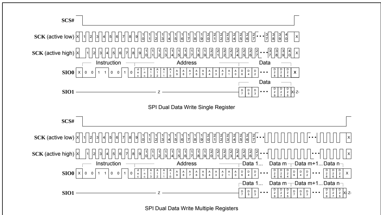
FIGURE 10-13: SPI DUAL DATA WRITE
