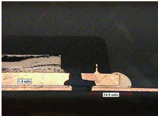
37% Paste Coverage, Plugged Via, 1.4 mil Standoff
