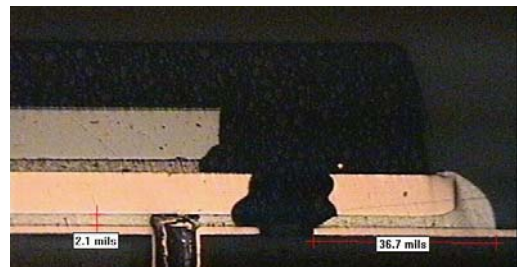
81% Paste Coverage, Encroached Via, 2.1 mil Standoff
