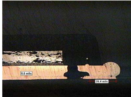
37% Paste coverage, Encroached Via, 0.6 mil Standoff
