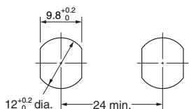
Note: The panel thickness is 1 to 3 mm.
