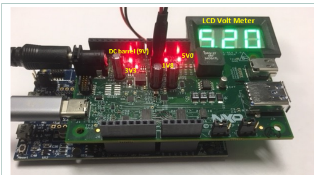
Figure 10. Shield 2 dock board control and LED indication
