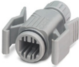
RJ45 sleeve housing, IP67, for pin insert VS-08-ST-RJ45, with push-pull interlocking for panel mounting frames, for cable cross section 5.0 mm ... 6.5 mm
