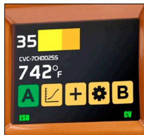
Tip temperature displayed on large color screen.
