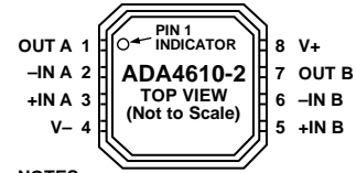
Figure 5. ADA4610-2 Pin Configuration, 8-Lead LFCSP_VD (CP Suffix)
