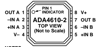
Figure 5. ADA4610-2 Pin Configuration, 8-Lead LFCSP_VD (CP Suffix)
