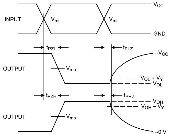
Figure 4. Switching Waveforms
