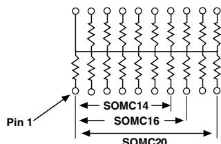
13, 15, or 19 resistors with one pin common
