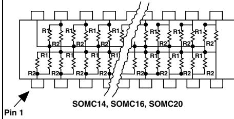
TTL dual-line terminator; pulse squaring, 12, 14, or 18 pairs of resistors
