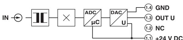
Figure 2 Block diagram for voltage output
