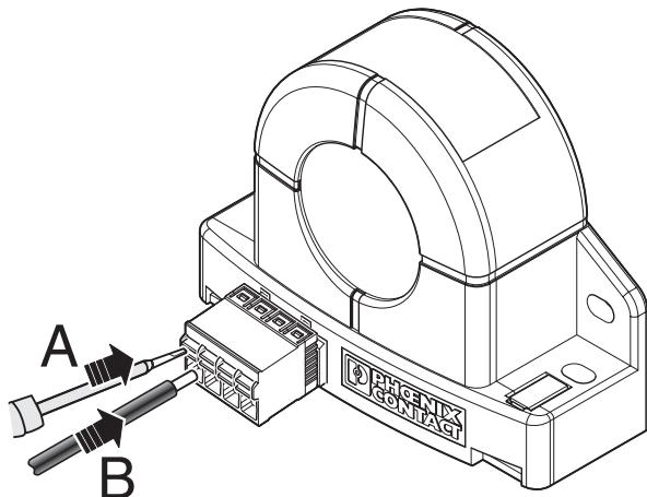
Figure 5 Spring-cage connection
