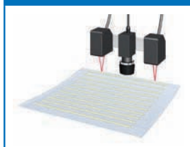
Inspecting Glass Heights (Autofocus)
