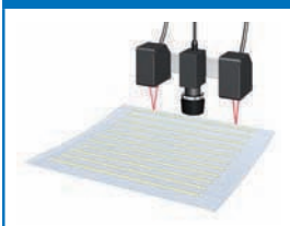
Inspecting Glass Heights (Autofocus)
