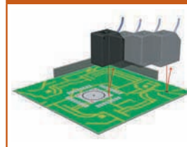
Inspecting Board Heights
