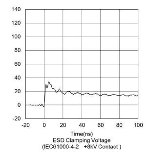
ESD Clamping Voltage VCL(V)
