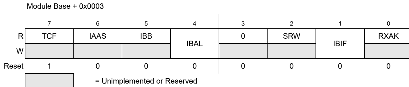
Figure 16-7. IIC Bus Status Register (IBSR)
