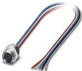
Bus system flush-type plug-in connector, socket, DeviceNet, 5-pos., M8, front/screw mounting with M10 fastening thread, with 0.5 m TPE litz wire, 5 x 0.25 mm 2
