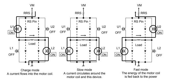
**Output transistor operational function**
